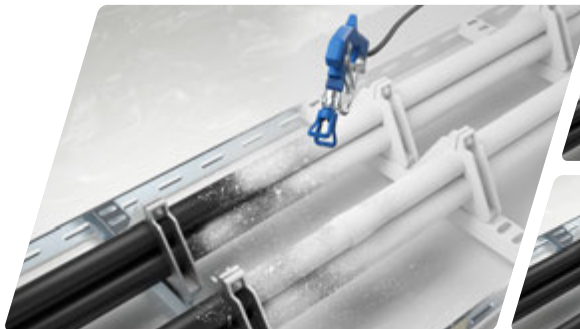
1. Coating with PYRO-SAFE® FLAMMOTECT-A can be carried out by means of airless painting (nozzle hole > 0.019 inch = 0.48 mm), taking into account the operating instructions of the airless unit.
